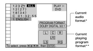
\* "PCM," "DTS" or "DOLBY DIGITAL" is displayed. In "DOLBY DIGITAL" case, the channels in the playing track are displayed by number as follows:
